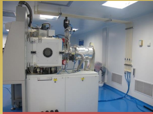
Multi source PVD with turbo molecular pump
